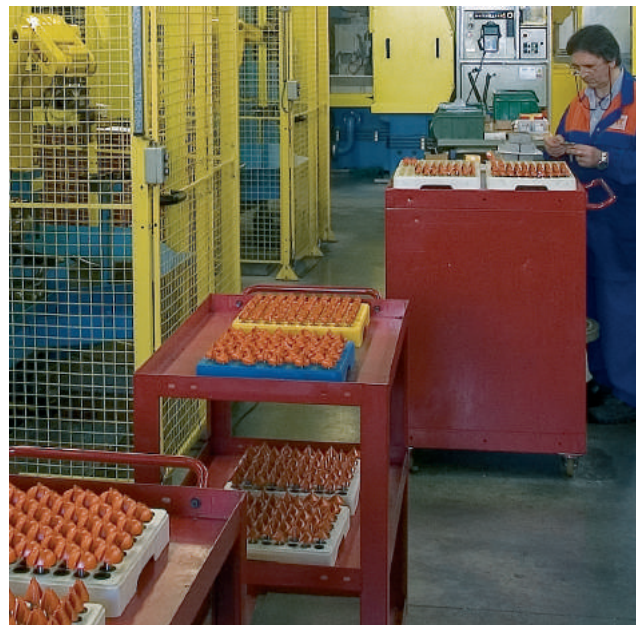
Loading the automated multi-axis CNC sharpening machines.
