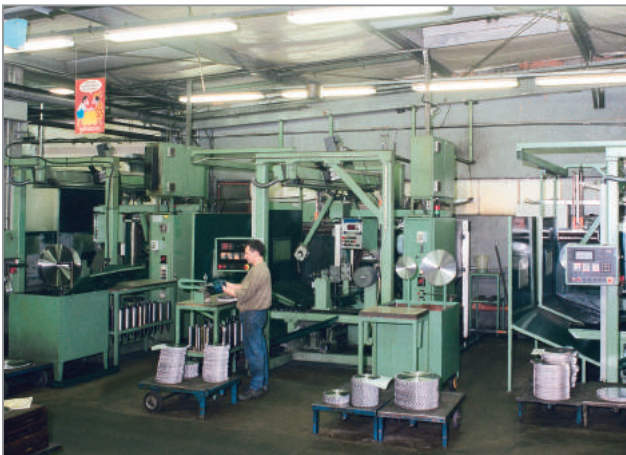
Grinding and tensioning the blades.
