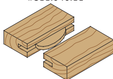
Biscuit joint using bit #811.040.11
